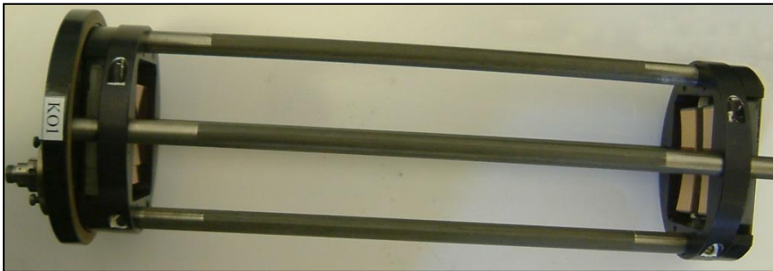
“Chernin” multi-pass analytical cell (25 cm * 156 passes = 39 m)
